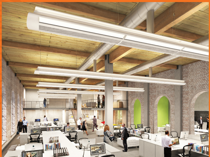
VENTUS LUX integrated service beams with incorporated LED lighting
