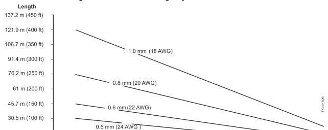
Figure 8: Maximum Wire Length by Current and Wire Size
