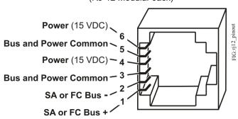
**Note:** Do not use the modular SA Bus port and the terminal block SA Bus simultaneously. Only use one of these connections at a time.
