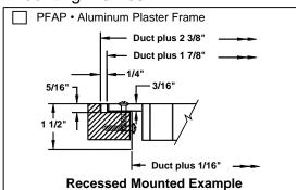
Note: Plaster frame can be installed as either surface mount or recessed. Note: Dimensions are in inches. Wall or duct opening should be duct sizes + 1/8.
