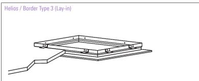
The Helios series of diffusers are not available with standard border type 1. For surface mounting applications, the TRM optional Rapid Mount frame can be used. Using border option TRM, the Helios series diffusers are shipped with border type 3 (lay-in). The TRM frame is shipped separate for field installation. Once the TRM is installed, the Helios diffuser simply lays into the frame. This option allows access into the ceiling after installation.
