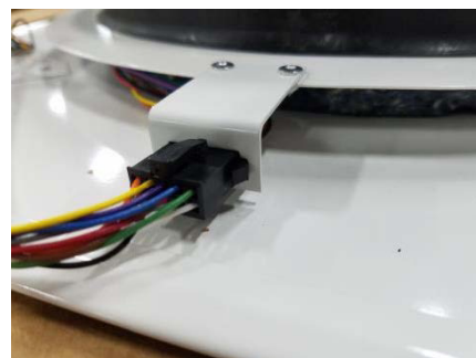
Figure 5. Plaque assembly wiring connection
