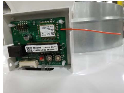
Figure 6. Control Board Enclosure
