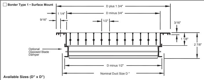
Border Type 1 is available in sizes 6" x 4" through 48" x 48" in one piece construction. Sizes larger than 48" x 48" are shipped in multiple sections with joining strips for field assembly. Odd and fractional sizes are available at additional cost.
