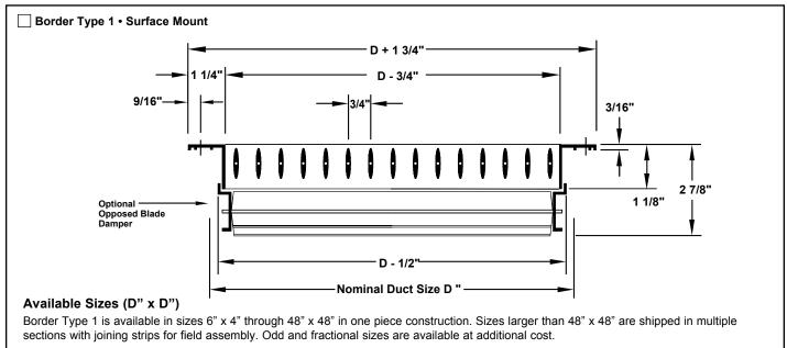
Note: Dimensions are in inches. Wall or duct opening should be duct size ± 1/8."
