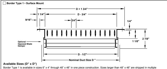
Border Type 1 is available in sizes 6" x 4" through 48" x 48" in one piece construction. Sizes larger than 48" x 48" are shipped in multiple sections with joining strips for field assembly. Odd and fractional sizes are available at additional cost.
