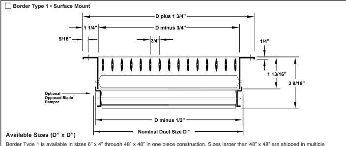
Border Type 1 is available in sizes 6" x 4" through 48" x 48" in one piece construction. Sizes larger than 48" x 48" are shipped in multiple sections with joining strips for field assembly. Odd and fractional sizes are available at additional cost.
