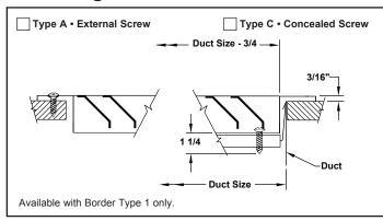
Note: Dimensions are in inches. Wall or duct opening should be duct size ± 1/8."
