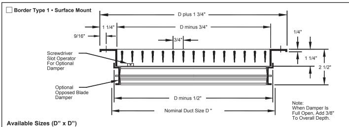
Border Type 1 is available in sizes 6" x 4" through 48" x 48" in 2" increments in one piece construction. Odd and fractional sizes are available at additional cost. Sizes larger than 48" x 48" are shipped in multiple sections with joining strips for field assembly.
