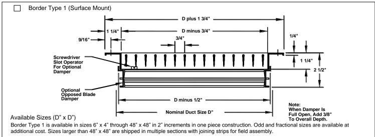
Note: Wall or duct opening should be duct area  $\pm 1/8$ ". All dimensions are in inches.
