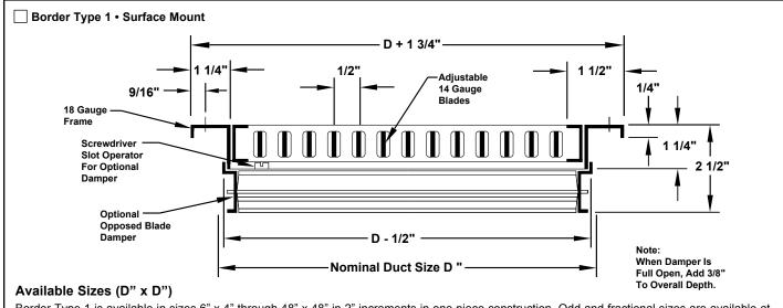
Border Type 1 is available in sizes 6" x 4" through 48" x 48" in 2" increments in one piece construction. Odd and fractional sizes are available at additional cost. Sizes larger than 48" x 48" are shipped in multiple sections with joining strips for field assembly.
