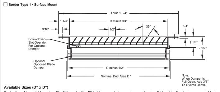
Border Type 1 is available in sizes 6" x 4" through 48" x 48" in 2" increments in one piece construction. Odd and fractional sizes are available at additional cost. Sizes larger than 48" x 48" are shipped in multiple sections with joining strips for field assembly.
