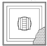
The pattern deflector in the neck of the diffuser consists of individually adjustable blades. These blades vary the discharge pattern from full horizontal to vertical and also damper the air volume. Square Neck • 4-Way (standard)
