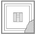
The standard Model PCS diffuser has a 4-Way discharge pattern. Also available are:
