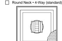
The pattern deflector in the neck of the diffuser consists of individually adjustable blades. These blades vary the discharge pattern from full horizontal to vertical and also damper the air volume.
