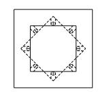
Pattern can be changed from side blow to corner blow and vice versa by removing four screws, rotating deflector 45 degrees, and replacing screws.
