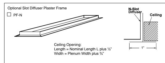
The PF-N diffuser mounting frame can be used in sheetrock or plaster ceiling. The frame is mounted in the ceiling by others. The Model N-1/N-4 diffuser is mounted on the inside lip of the frame. Plaster frame is 1 1/2" in height.
