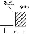
The PF-N diffuser mounting frame can be used in sheetrock or plaster ceiling. The frame is mounted in the ceiling by others. The Model N-1-D/N-4-D diffuser is mounted on the inside lip of the frame.
