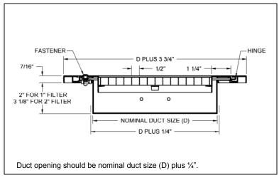
Side Cross-Sectional View: Border Type 1 (Surface Mount) & Border Type 3 (Lay-in T-Bar)
