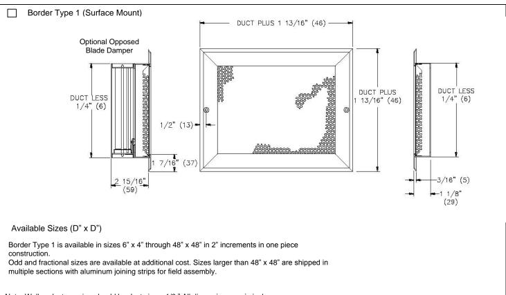
Note: Wall or duct opening should be duct size  $\pm$  1/8." All dimensions are in inches.
