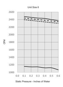
No Coil or with Electric Coil 1 Row Water Coil - - - -2 Row Water Coil -----
