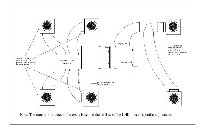
In a neutral plenum, the supply can be ducted with the induced air inlet open to the plenum. Once again, the discharge would be flex ducted to TAF-R's. Both of these layouts can be used in a conference room to boost the air supplied.
