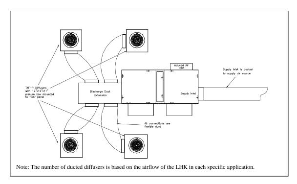
The LHK can also be used for perimeter applications. The LHK would use the TAF-D, a CT linear bar grille with attached plenum box, as supply grilles and as returns. The returns would be ducted back to the LHK induced air inlet. The supply would be ducted back to the supply air source.
