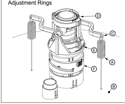
Control disc springs (A) must be disconnected from control disc (B) to ensure that the diffuser is in the fully open position for commissioning purposes.
