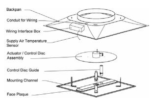
Master diffusers are created by connecting the  $T_3SQ$  -1 diffuser to a wall mounted controller / thermostat using the blue RJ-45 control cable.  $T_3SQ$ -1 drone diffusers are created by connecting the diffuser to a master unit using the blue RJ-45 control cable.
