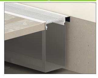
Cross section view of an installed TAF-L-R
