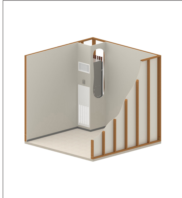
Figure 110. Typical Vertical Stack Application
