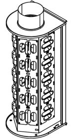
View showing integral variable air pattern controllers
