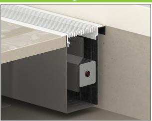
Cross section view of an installed TAF-L-W
