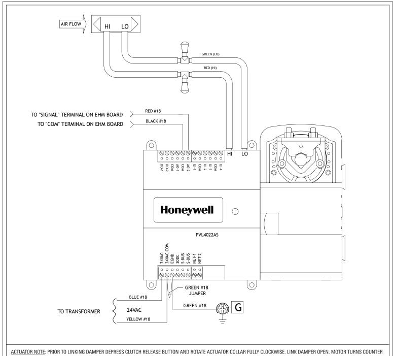
ACTUATOR NOTE: PRIOR TO LINKING DAMPER DEPRESS CLUTCH RELEASE BUTTON AND ROTATE ACTUATOR COLLAR FULLY CLOCKWISE. LINK DAMPER OPEN. MOTOR TURNS COUNTER CLOCKWISE TO CLOSE.
