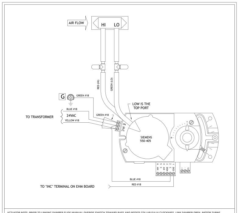
ACTUATOR NOTE: PRIOR TO LINKING DAMPER SLIDE MANUAL OVERIDE SWITCH TOWARD BASE AND ROTATE COLLAR FULLY CLOCKWISE. LINK DAMPER OPEN. MOTOR TURNS COUNTER CLOCKWISE TO CLOSE. SLIDE MANUAL OVERIDE SWITCH BACK TO ORIGINAL POSITION.
