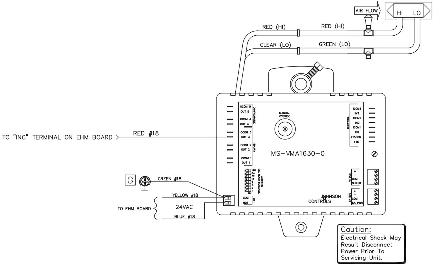
**ACTUATOR NOTE:** PRIOR TO LINKING DAMPER DEPRESS MANUAL OVERRIDE BUTTON AND ROTATE ACTUATOR COLLAR FULLY CLOCKWISE. LINK DAMPER OPEN. MOTOR TURNS COUNTER CLOCKWISE TO CLOSE.
