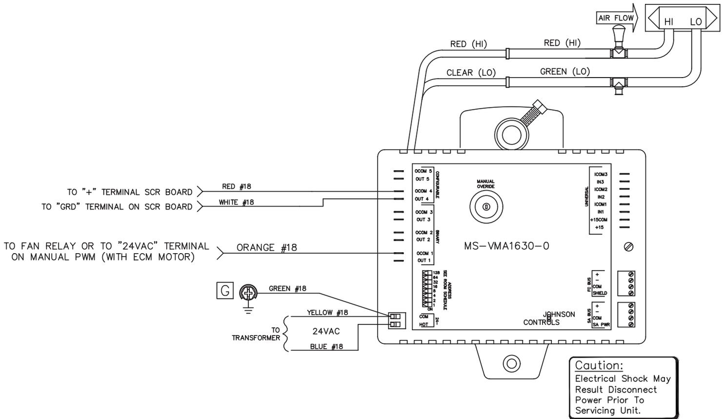
ACTUATOR NOTE: PRIOR TO LINKING DAMPER DEPRESS MANUAL OVERRIDE BUTTON AND ROTATE ACTUATOR COLLAR FULLY CLOCKWISE. LINK DAMPER OPEN. MOTOR TURNS COUNTER CLOCKWISE TO CLOSE.
