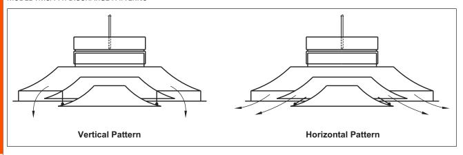
Note: Pattern controller vanes are adjustable to provide vertical or horizontal airflow
