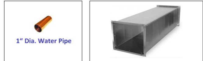
Figure 1: Cooling energy transport capacity of water versus air
