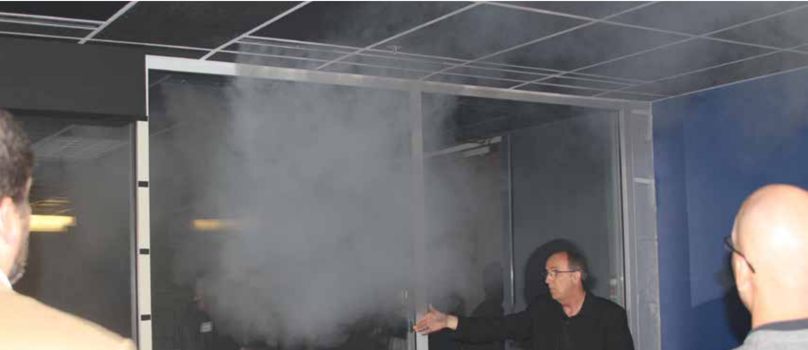
Above: Jim Aswegan, Chief Engineer, displays the air pattern of the solar-powered EOS diffuser. Below: Smoke tests of various Titus products.
