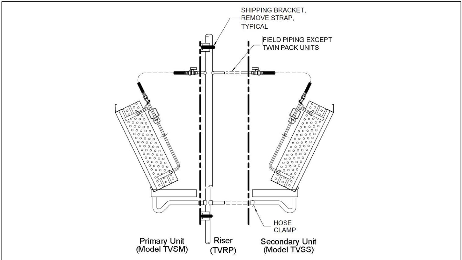
**FACTORY FURNISHED -FIELD INSTALLED RISERS (Shipped Loose Riser)**
