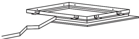
The Helios series of diffusers are not available with standard border type 1. For surface mounting applications, the TRM optional Rapid Mount frame can be used. Using border option TRM, the Helios series diffusers are shipped with border type 3 (lay-in). The TRM frame is shipped separate for field installation. Once the TRM is installed, the Helios diffuser simply lays into the frame. This option allows access into the ceiling after installation.
