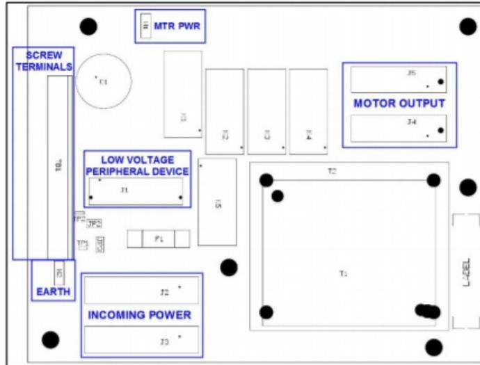
**Figure 2 – Connector Layout**
