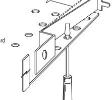
3. Face will swing down. For complete removal, remove pivot pin.
