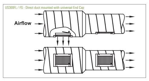
Application Note: For duct velocities up to 800 fpm, the damper/extractor is not required. For duct velocities higher than 800 fpm, the damper/extractor is recommended.
