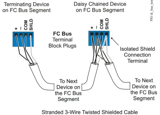
**Note:** The Shield terminal (SHLD) on the FC Bus terminal block is isolated and can be used to connect the cable shields on the bus ([Figure 3](#)).
