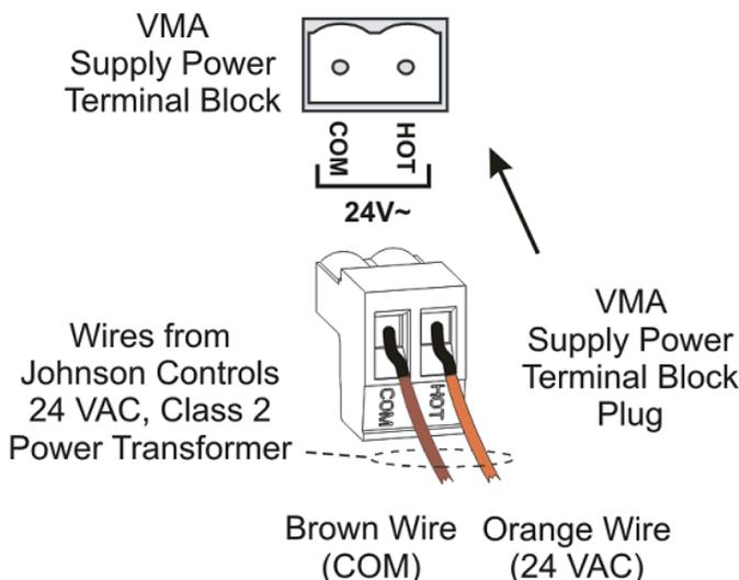
**Important:** Connect 24 VAC supply power to the VMA and all other network devices so that transformer phasing is uniform across the network devices. Powering network devices with uniform 24 VAC supply power phasing reduces noise, interference, and ground loop problems. The VMA does not require an earth ground connection. However, when grounding the secondary of the 24 VAC transformer is required, only one connection to ground should be made near the transformer. See the following figure.
