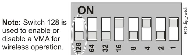
To set the device addresses on a *Metasys* field controller:
