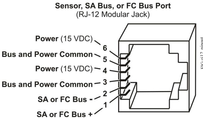
**Note:** Do not use the modular SA Bus port and the terminal block SA Bus simultaneously. Only use one of these connections at a time.
