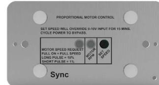
ECM motors shipped with remote PWM controller require a signal from the DDC controller to control fan speed.
