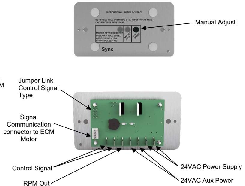
The Manual PWM interface board allows accurate manual adjustment and monitor of fan with the GE Electric ECM Motor.
