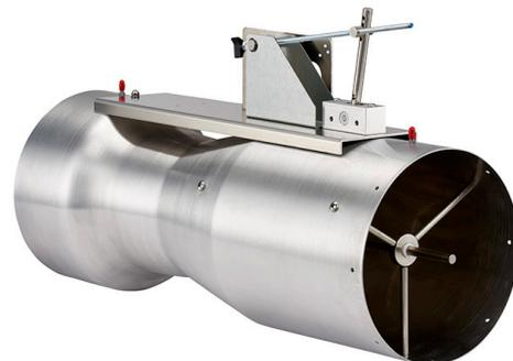
Constant volume (CV) Venturi Air Valves provide a single CFM set point for applications that require only one air flow set point. CV valves do not come with a controller or actuator.
