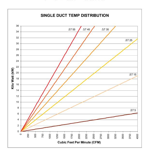
The most important criteria for selecting kW is diffuser mixing performance and thermal comfort. The ASHRAE Fundamentals Handbook, Chapter 31, states discharge temperature to the space should not exceed 15°F above the desired room temperature for thermal comfort. For a typical application where the space temperature is 75°F, the maximum discharge temperature would be 90°F.
