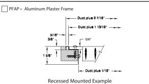
Note: Wall opening should be listed duct size + 1/s" to listed duct size + 1/s".
