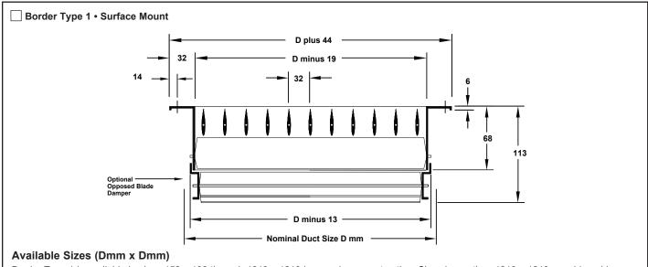
Border Type 1 is available in sizes 152 x 102 through 1219 x 1219 in one piece construction. Sizes larger than 1219 x 1219 are shipped in multiple sections with joining strips for field assembly. Odd and fractional sizes are available at additional cost.
