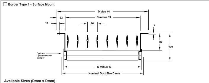
Border Type 1 is available in sizes 305 x 305 through 1219 x 1219 in one piece construction. Sizes larger than 1219 x 1219 are shipped in multiple sections with joining strips for field assembly. Odd and fractional sizes are available at additional cost.
