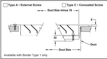
Note: Dimensions are in millimeters. Wall or duct opening should be duct size ± 3.
