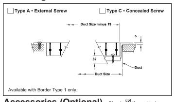
Note: Dimensions are in millimeters. Wall or duct opening should be duct size  $\pm$  3.
